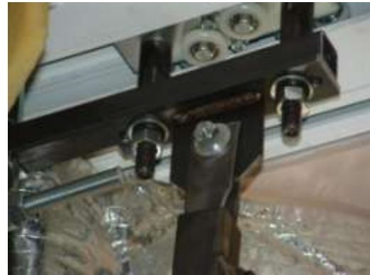
Figure 8.1. Attaching Stabilizer Bar to Trolley
