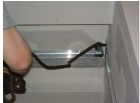
Figure 3.5.a. “Threading” End Sprocket Assembly
