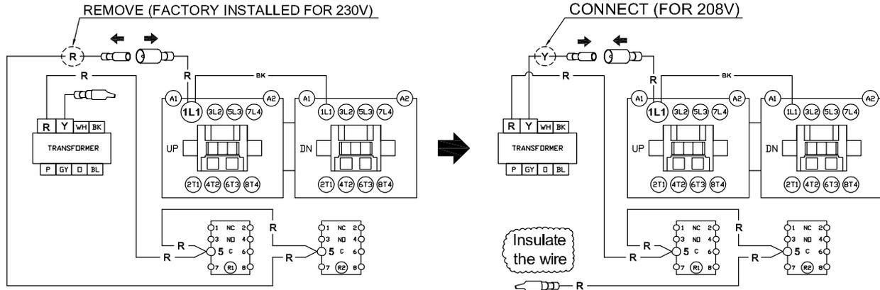
1. Unplug the red "230V" wire connector from the red "PWR" wire connector.
