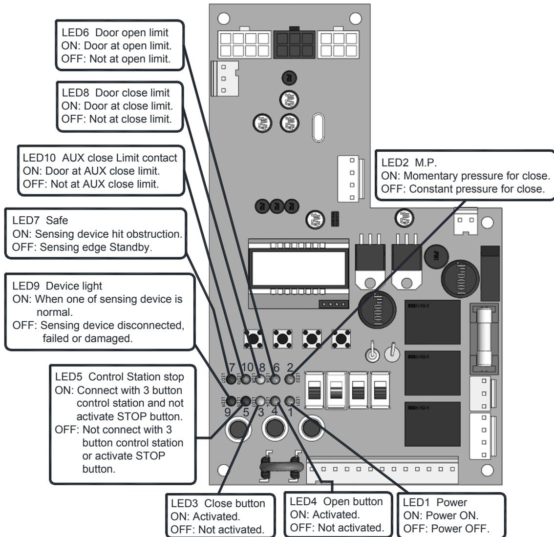
FGH 208V/230V 3 PHASE 50/60HZ LH (FGEP BOARD)
