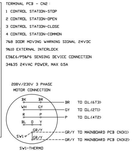
FGH 460V 3 PHASE 50/60HZ LH (FGEP BOARD)
