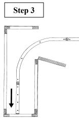
**Step 1.** Install track curves (if applicable) or straight track at storage pockets first. Maintain clearance for the folded grille by measuring at least 4" to the <u>outside</u> of the track. See illustration.
