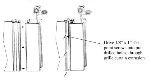
**Step 3.** Connect lock posts to the grille curtain sections after they are hanging from the track. (See illustration at left).
