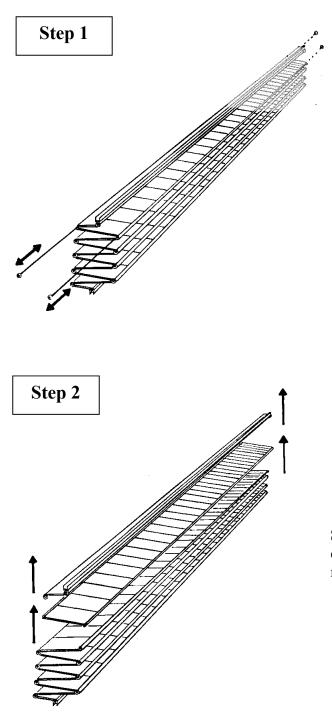
**Step 1.** Take a #2 square (Robertson type) screwdriver and clamp with vise-locking pliers to give the driver leverage. Use this driver to hold the screw at the end of a hinge rod while unthreading the other end. Remove the hinge rods on each side of the panels that you wish to remove.
