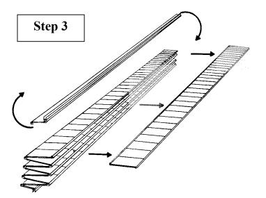
**Step 3.** If you have removed an <u>even</u> number of panels, then lower the half panel and connecting hinges straight down onto the remaining panels. If you have removed an <u>odd</u> number of panels, then you must rotate the half panel with it's connecting hinge end-forend for 180 degrees and lower it onto the remaining panels.
