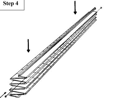
**Step 4.** Line up hinge components, replace the hinge washers and screws. Tighten by reversing Step 1.
