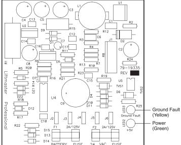
Figure 1 - Logic Board LED Descriptions
