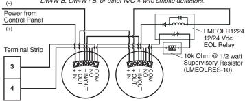
FIGURE 5 NOTE: Follow this method of attachment when using LM1424, LM1412, or other N/O 4-wire smoke detectors. (+)
