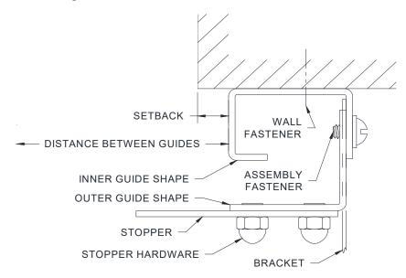
Figure 5.1 – UL9 Face of Wall Guide without Brush
