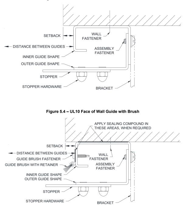
Figure 5.3 – UL10 Face of Wall Guide without Brush
