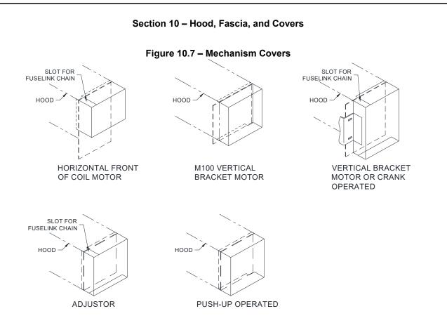
**Note:** Mechanism covers differ from operator and adjustor covers in that operator and adjustor covers provide a complete enclosure.
