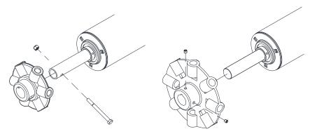
Figure 6.2 – Removal of Adjustor From Barrel Assembly
