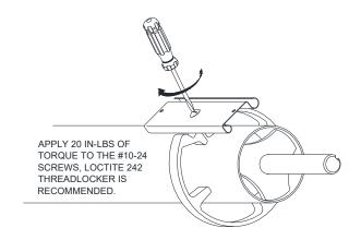
Figure 8.2 - UL-9 Fastening Section Attachment
