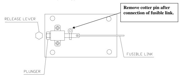
**NOTE:** Fusible link release can be substituted by alarm release box. Fusible link release can be removed by loosen the 2 screws. Alarm release can be attached by using the 4 screws.
