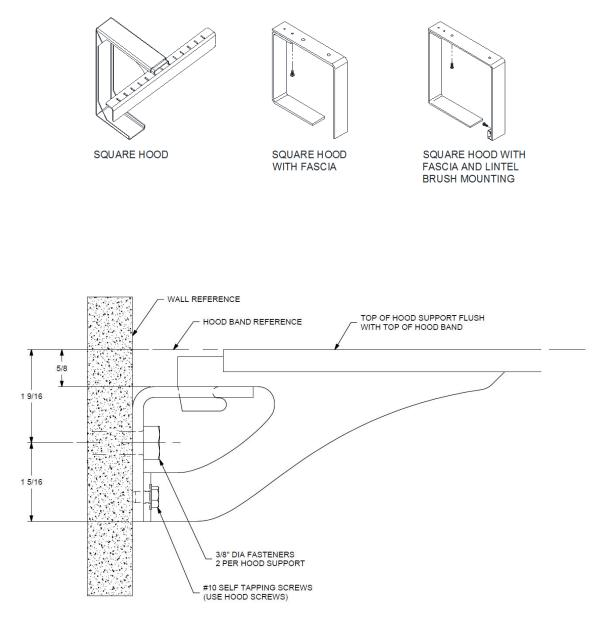
**Note:** See above detail for face of wall units; the wall angle is offset 5/8" from top of hood band to allow hood support to be flush while installing the hood.
