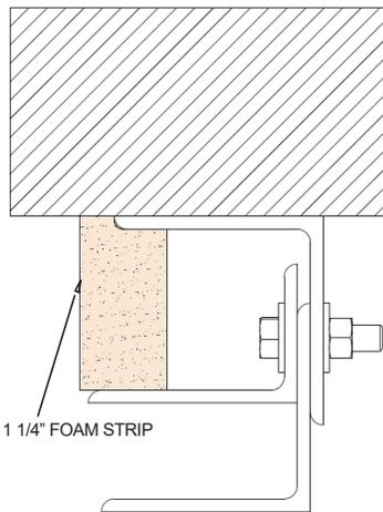
Sound Transmission Class (STC) rating is 27 for a full door when configured with 18GA steel front slats. Please contact the factory for details.
