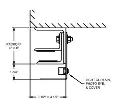
**FACE OF WALL – Z GUIDE** Typically used with masonry wall construction
