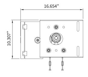
The indirect splash-proof MG operator comes with a totally enclosed non-ventilated (TENV) motor, NEMA 4 control box and powder coated steel mounting plates.
