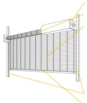
**BRACKETS**- Steel with SpectraShield® powder coating in Gray. Bolt to guide assembly and support counter-balance shaft and curtain.
