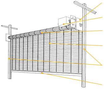
**BRACKETS** - Steel with powder coating in Gray. Bolt to guide assembly and support counter-balance shaft curtain.
