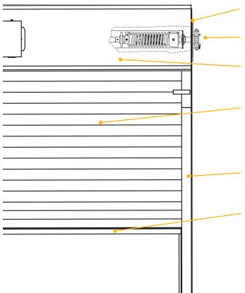
**BRACKETS** - Steel with powder coated finish to match curtain. Bolt to guide assembly and support counter-balance shaft and curtain.
