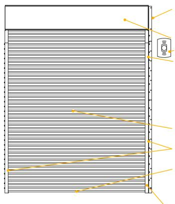
**BRACKETS** - Steel with powder coated finish to match curtain. Bolted to guide assembly and support counter-balance shaft and curtain.
