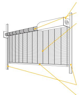
**BRACKETS**- Steel with SpectraShield® powder coating in Gray. Bolt to guide assembly and support counter-balance shaft and curtain.
