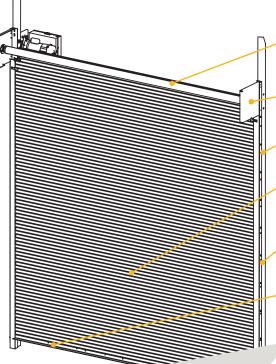
**COUNTER-BALANCE SHAFT** - Hidden above the ceiling, it is made of steel. It supports the curtain and contains torsion springs for assisting operation.
