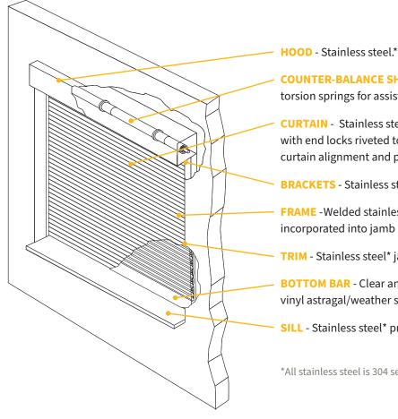
**COUNTER-BALANCE SHAFT** - Steel.\* Supports curtain and contains torsion springs for assisting operation.
