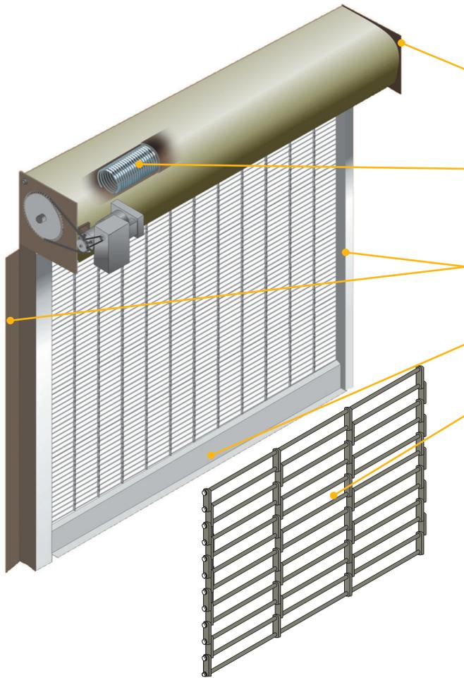
**BRACKETS** - Steel with powder coating in Gray. Bolt to guide assembly and support counter-balance shaft and curtain.
