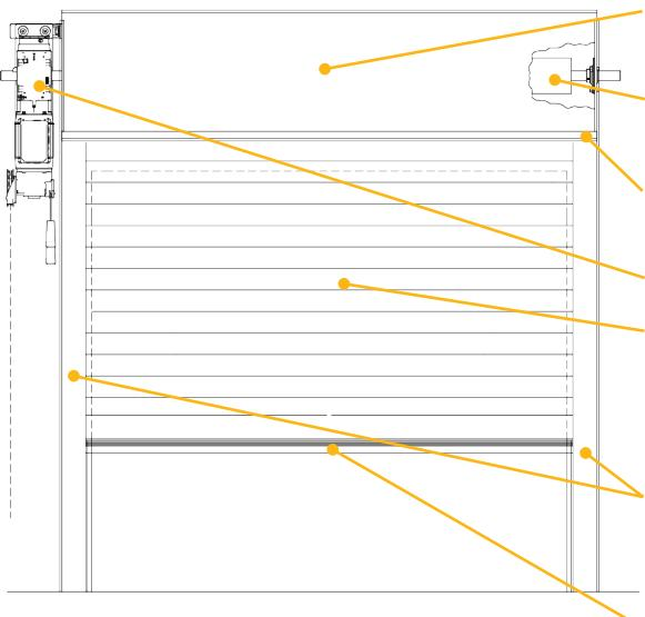
**HOOD** - Galvanized steel with powder coat finish to match curtain. Encloses the curtain and provides weather resistance at the head of the door.
