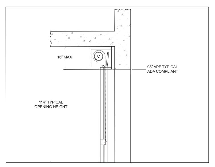
The Extreme High Performance MicroCoil Grille -500K Cycles was designed with parking in mind. One of every six accessible parking spaces must be ADA van accessible in a parking garage. Since an ADA van only clears a typical opening of the parking structure by ~16", installing a security grille used to be quite the challenge.
